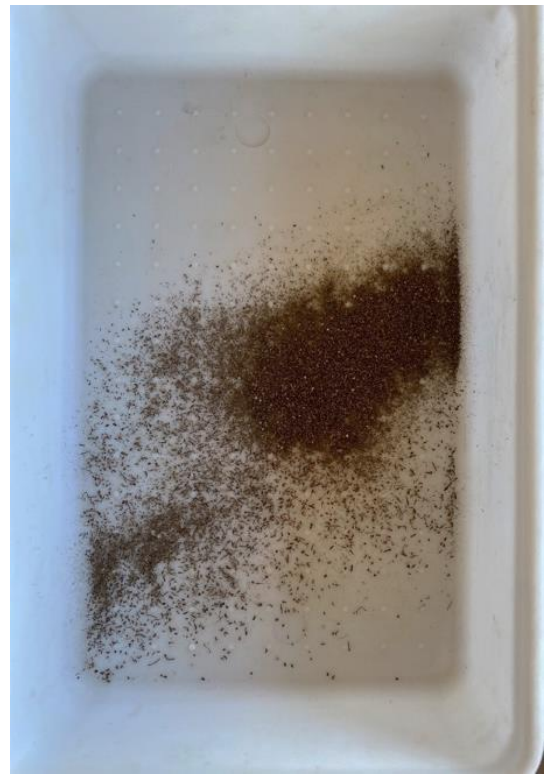
Figure 7. Soil passed through 2-mm sieve.
