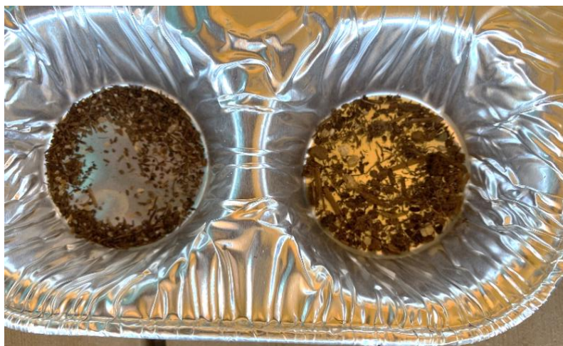
Figure 15. Coarse material sand, roots, etc. collected by dry sieving that is the same size as the aggregates and need to be separated from the measurements of aggregates before drying for 1-2 mm (left) and >2 mm aggregates (right).
