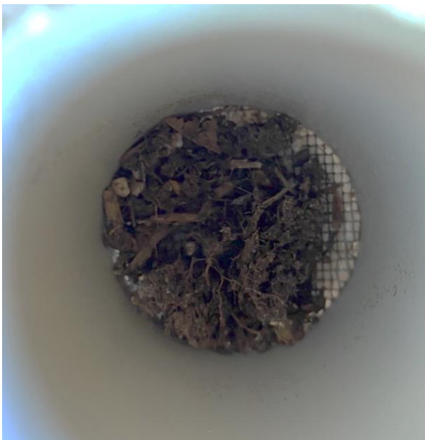
Figure 8. Soil left in 2mm sieve after shaking
