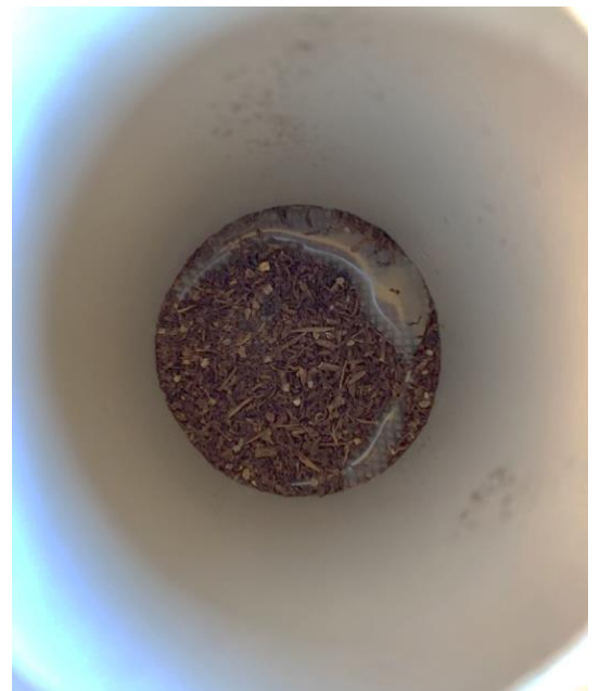
Figure 9. Soil passed through 2-mm sieve was placed on 1-mm mesh.
