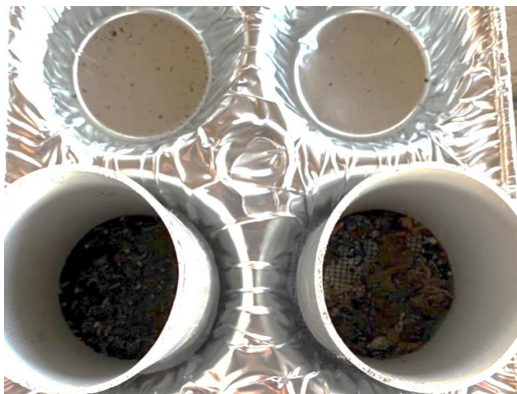
Figure 12. Soil passed through the mesh after capillary rewetting (top) and water-stable aggregates on the mesh after wetting sieving (bottom) for 1-2 mm (left) and >2 mm aggregates (right).
