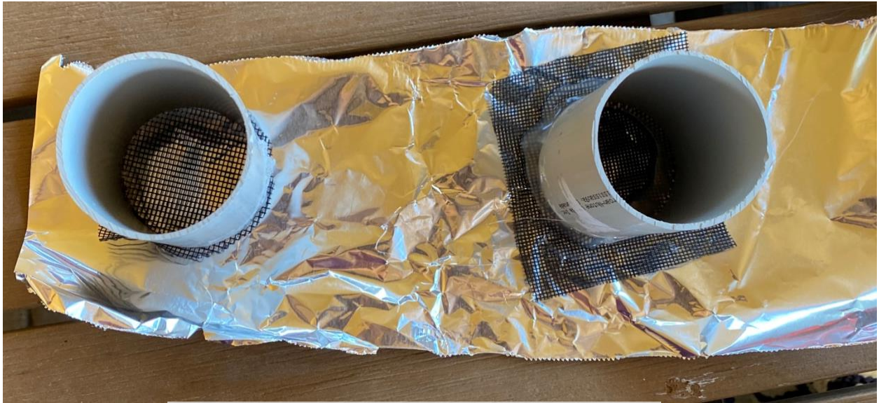
Figure 3. Gluing mesh to PVC pipe on foil
