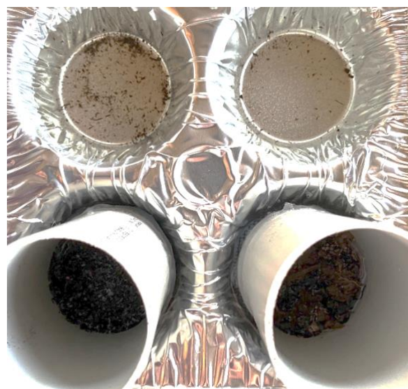
Figure 13. Soil particles in unstable aggregates passed through the mesh (top) and water-stable aggregates were broken up to collect coarse material (bottom) for 1-2 mm (left) and >2 mm aggregates (right).
