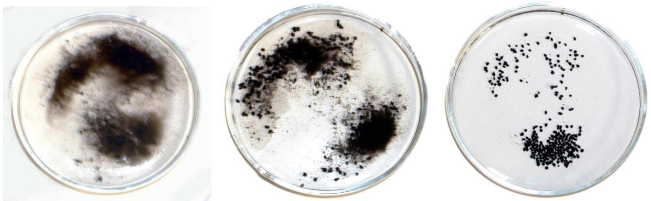
Figure 16. The 1-2 mm aggregates in the picture on the left were 14% water stable while those in the center were 47% stable and on the right were 93% stable.
